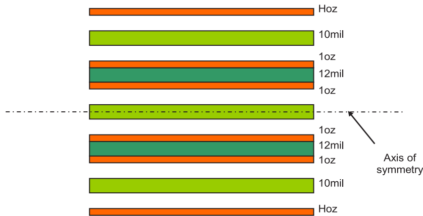
Figure 2: Symmetrical board layer design.
