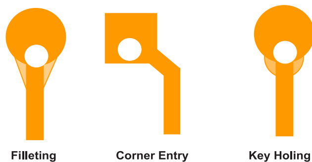
Figure 14: Connections between the trace and holes.
