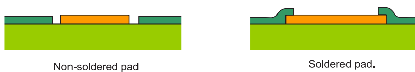
Figure 22: Solder mask openings for copper pads.
