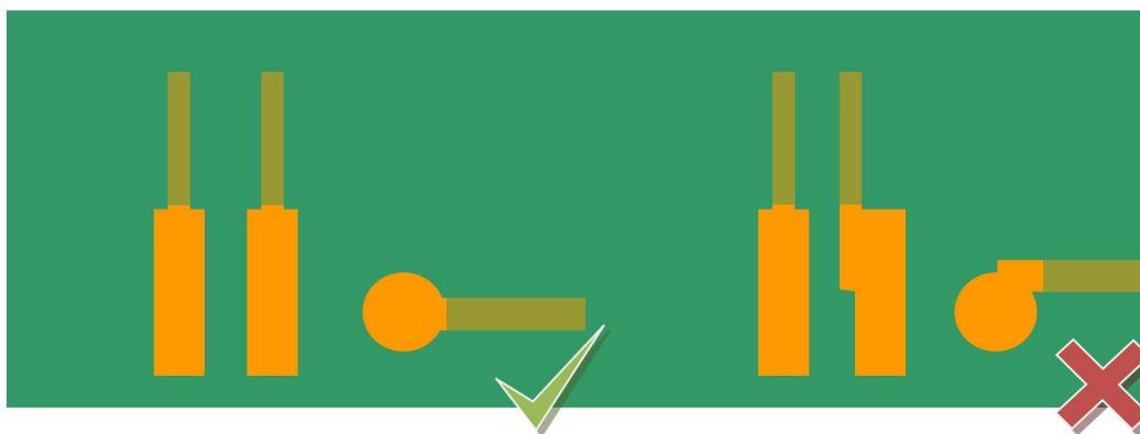
Figure 11: Poor trace and pad alignment.
