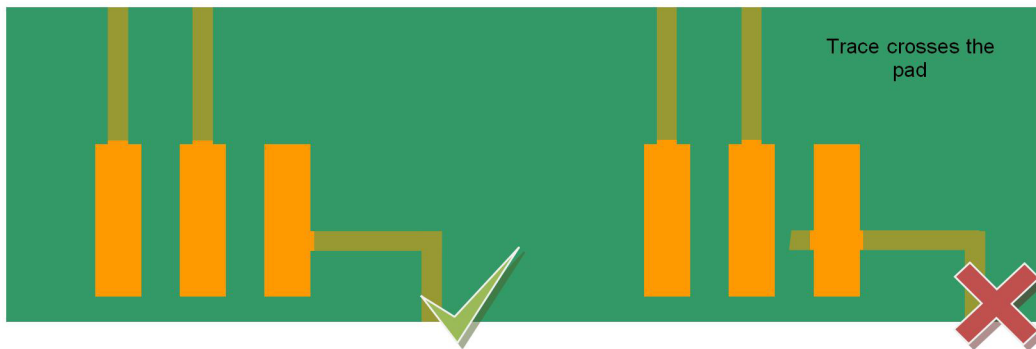
Figure 10: Starting position of the trace to the pad.
