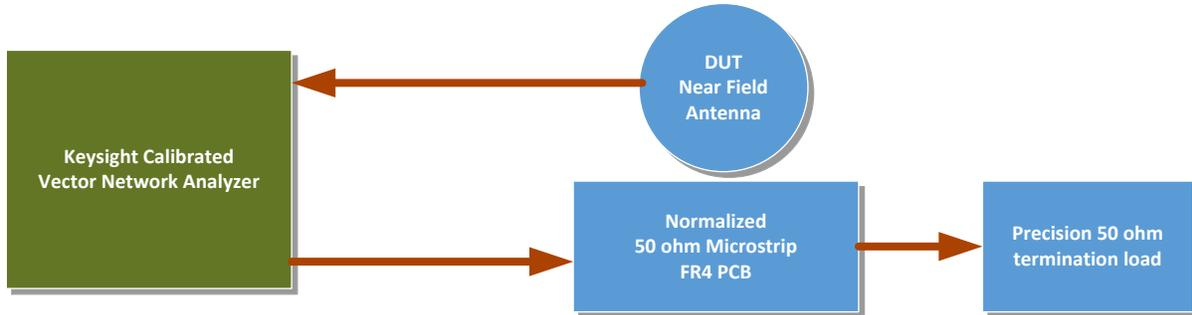
The antenna must be vertical 90 degrees against PCB signal trace, at 0mm distance, parallel horizontal orientation to signal trace for maximum sensitivity of the magnetic flux, as depicted below.
