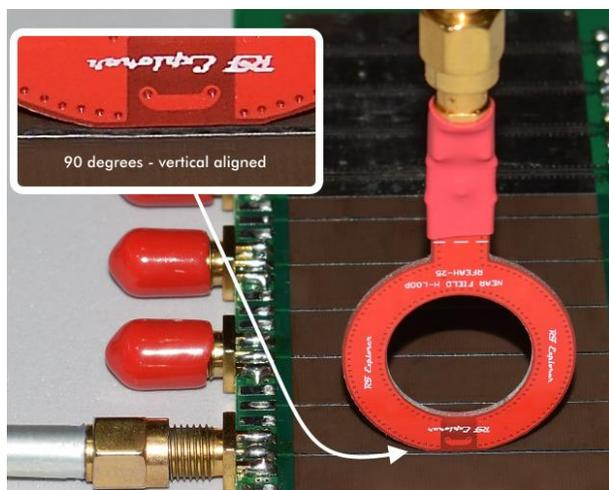
The H-Loop antenna works basically as an inductive coil, capturing magnetic flux. Therefore, it should be oriented in such a way the maximum magnetic field is captured.
