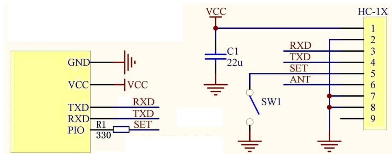
Please set the "SET" control pin to high level or hanging out in normal times, and set to low level in setting parameters state.
