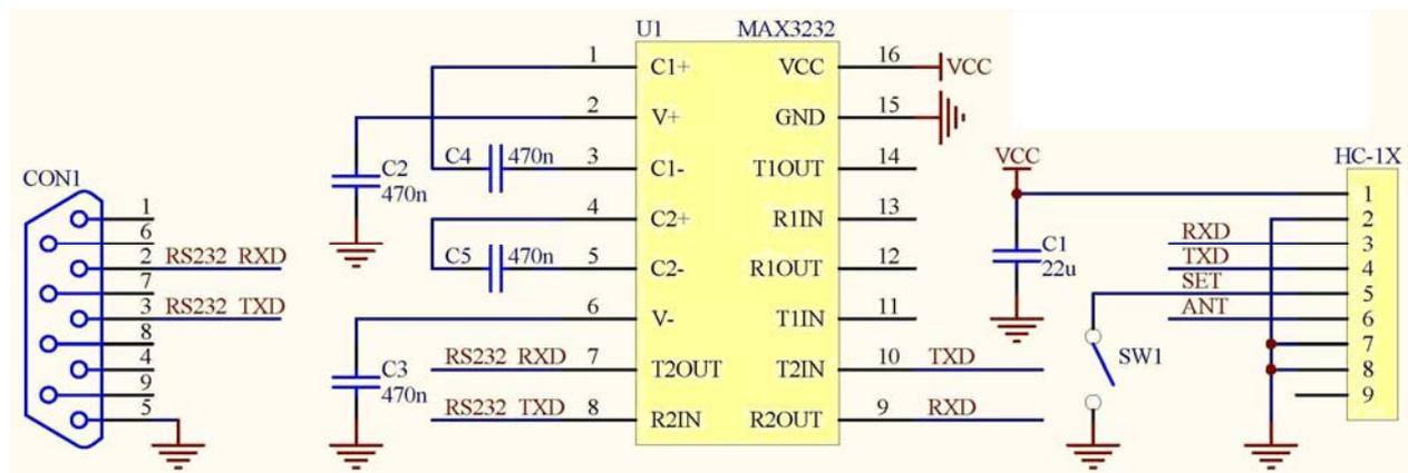
"SET" pin through the switch SW1 grounding can enter the parameter setting state, left hanging out.
