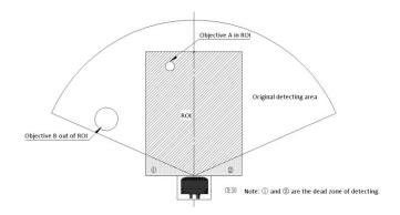
Figure 10 Schematic of ROI Function Determination
