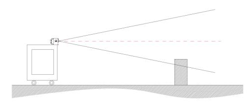
Figure 5 Application in the obstacle avoidance mode. Compared with the 2D Scanning LiDAR (the red line), CE30-A can detect obstacles lower than the mounting height.
