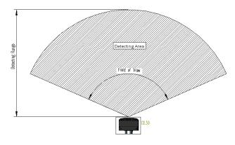
Figure 6 Illustration of Detecting Range and Area
