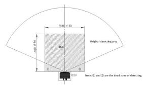
Figure 9 Schematic Diagram of ROI Function Description
