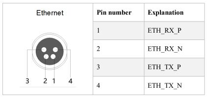
Figure 14 Ethernet Socket Pin Definition
