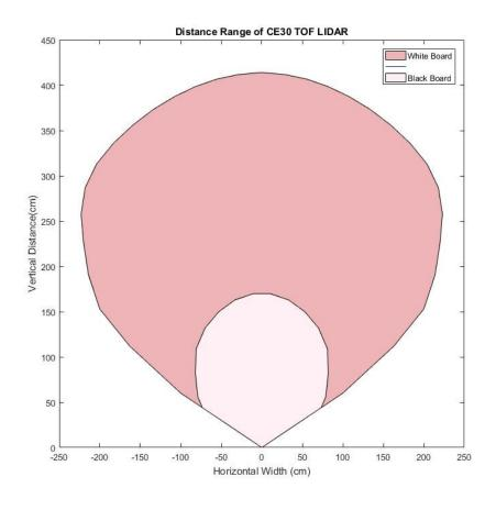
Figure 7 Optimized Detecting Area for Obstacle Avoidance Application
